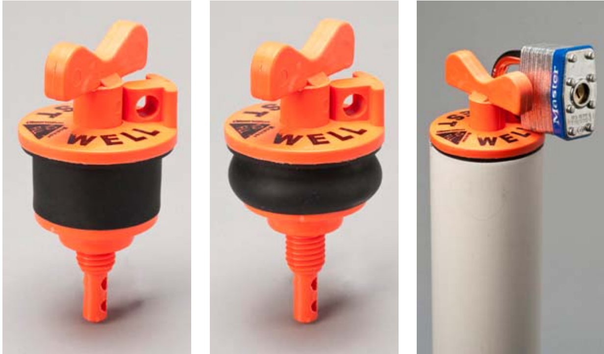
Caption: This locking plug for groundwater monitoring wells is molded in glass-filled nylon by Koby Environmental, Inc. Without a lubricant additive, friction would be so high at the surface that it would be very difficult to turn the wing nut, which creates the plug's seal (above, center). To reduce the coefficient of friction, Koby Environmental has chosen a Dow Corning® Siloxane Masterbatch from Multibase, Inc. Koby adds 2% by weight of the masterbatch, which itself is a 50% concentration of ultra-high-molecular-weight polydimethylsiloxane in a thermoplastic matrix.
